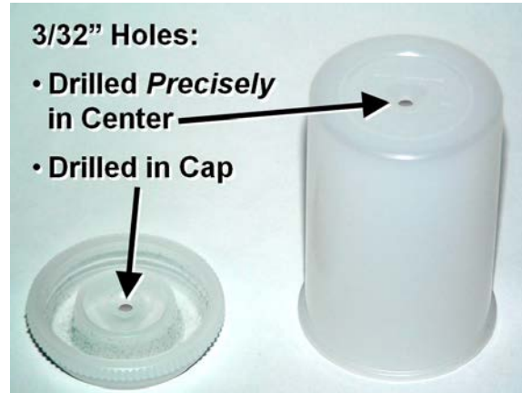
Figure 2.2-1: Holes Drilled in Thruster Housings
