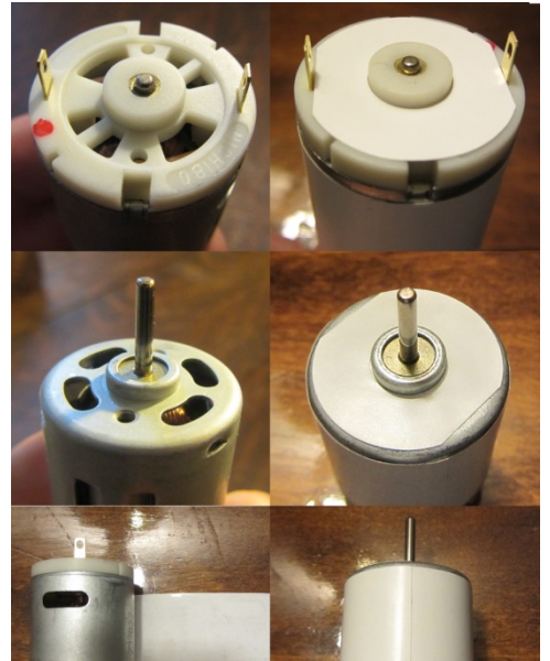
Figure 2.1-1: Motor Taping Process
