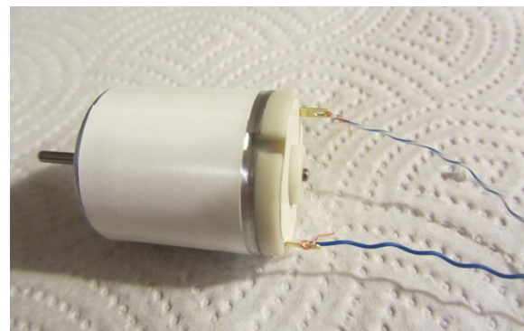
Figure 2.3-6: Tether Cable Wires Soldered Onto a Thruster Motor's Terminals
