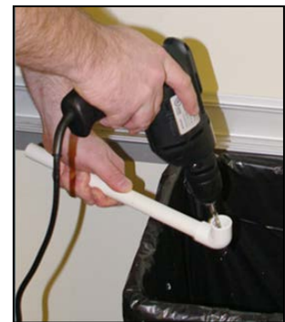
Figure 1.2-1: Drilling Elbow Hole over a Wastebasket
