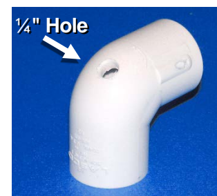
Figure 1.2-2: Drain Hole Drilled in a PVC Elbow
