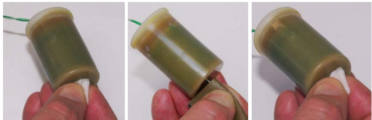
Figure 2.5-1: Cleaning, Roughening, and Re-cleaning a Motor Shaft
