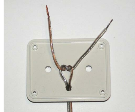
Figure 3.4-1: Power Cord Passed Through the Hole in the Box Lid, and Knotted
