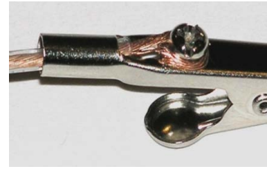
Figure 3.2-2: Wire Properly Connected to an Alligator Clip Screw
