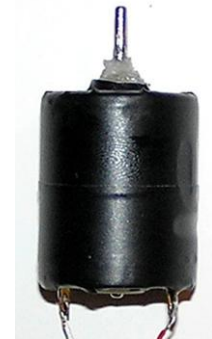
Figure 2.6-4: Petroleum Jelly Placed at the Base of a Motor's Shaft
