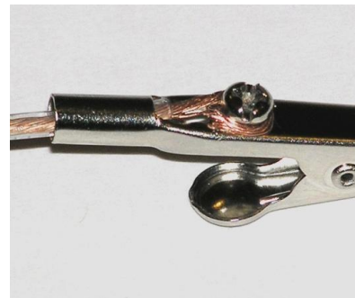
Figure 3.3-4: Wire Properly Connected to an Alligator Clip Screw
