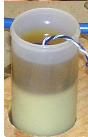
Figure 2.6-7: Wax Filled to 1/2" from the Top of the Housing
