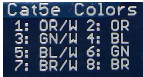
Figure 3.2-4: Connector Wire-Color Sequence Printed on the PCB
