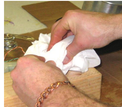
Figure 2.6-11: Using a Paper Towel While Placing the Cap on the Thruster Housing Can Help Prevent Wax from Squirting Onto You or Others
