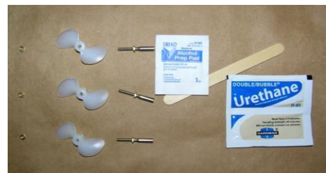
Figure 2.7-2: Propeller Parts, Ready to Assemble
