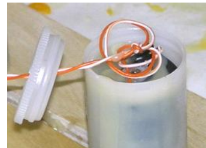
Figure 2.6-8: Wires Coiled in the Top of the Housing, Prior to the Final Wax Pour
