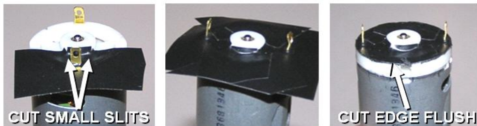
Figure 2.3-2: Tape Wrapping Process for the “Terminal” End of a Motor
