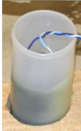
Figure 2.6-6: Motor Sealed in the Bottom of a Thruster Housing
