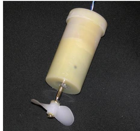
Figure 2.7-1: Propeller Mounted on a Motor's Shaft
