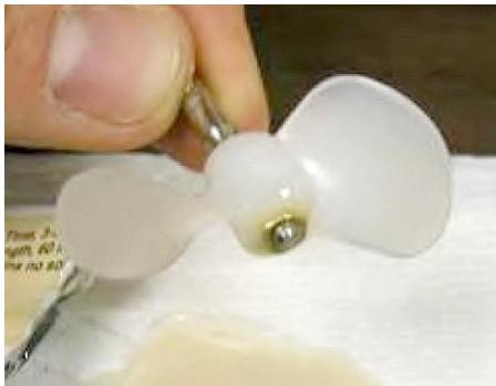
Figure 2.7-7: Nut Threaded Onto Shaft Coupler and Covered with Epoxy
