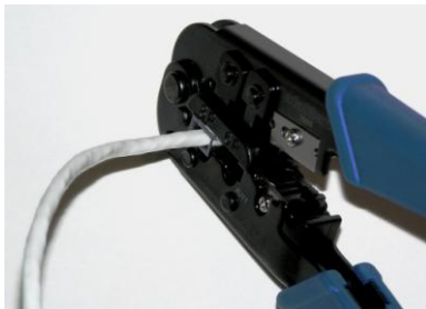
Figure 3.2-8: RJ45 Connector Plug in the Crimping Tool Cavity
