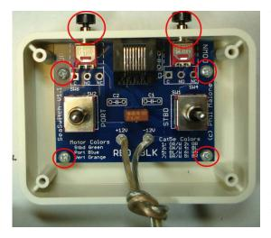
To test for shorts, connect your meter probes to the two alligator clips (red to red, black to black). At no time should you get a low resistance reading (continuity).
