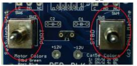
Your two toggle switches may look different than in this picture (they may have green cases) but they will operate the same. The switches must be firmly down and completely vertical when soldered. The best way to ensure this is to drop the box cover over the switches, and screw on the retaining nuts. This will ensure they will line up properly for final assembly.
