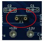
This is the smallest part, and it goes on first, in the middle of the board. The location is labeled F1. Put the socket pins in the two holes, and flip the board over while holding the socket in place.
