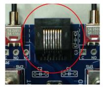
The final component is the socket for the tether. When attaching this to the board, insert the metal pins in the holes **first**, and then snap in the plastic retaining clips. Once the connector is in place, verify that all the pins are through the holes BEFORE soldering.
